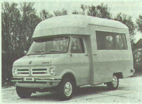
Left: Bedford Bedouin, looking forward. Note the Luton head storage space over the cab and the picture windows. Above: Exterior of the Bedouin.
