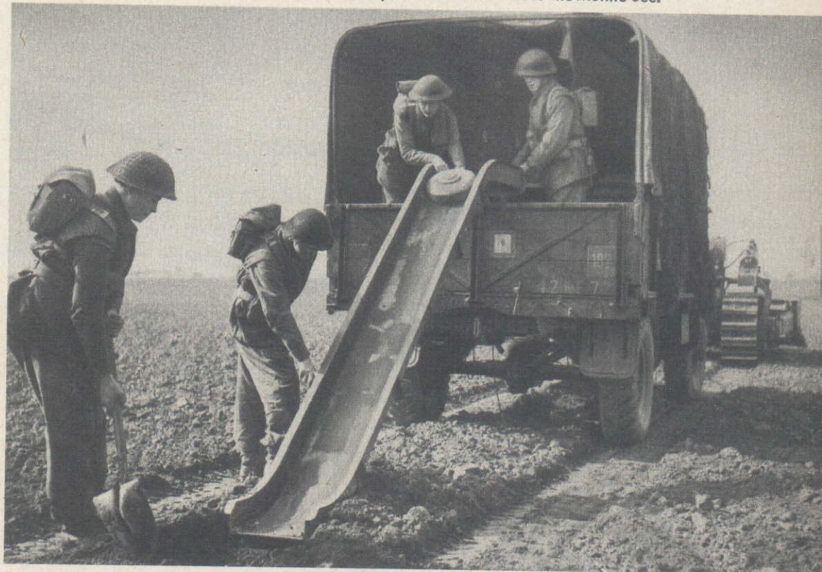
Like a farmer's mechanical seed-sower, this vehicle drops concrete mines into holes scoured by a bulldozer's grab. Sappers conceal the mines and the wheel tracks.
