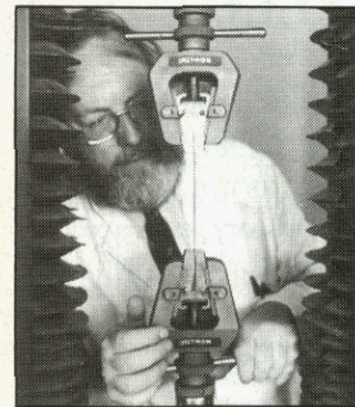
Senior scientific officer Don Scofield tests the breaking performance of stretch wrapping
