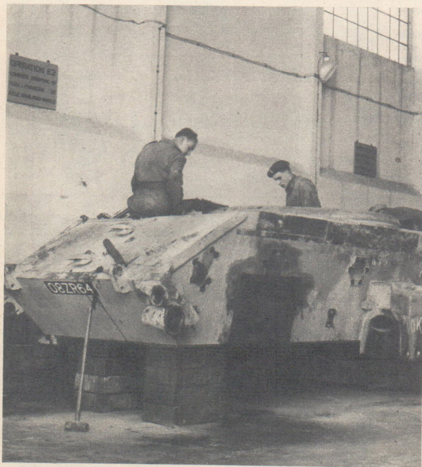
After removing tracks, wheels and axles British soldiers strip the hull of all its parts.
