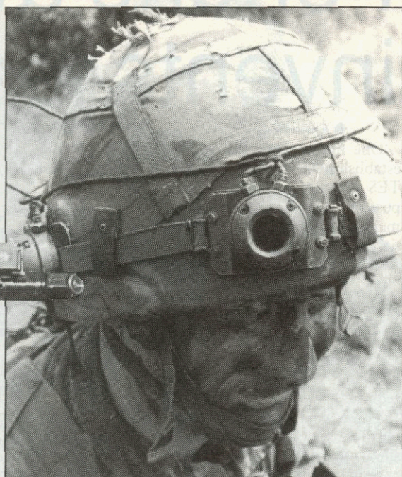
Left - An American soldier kitted up for laser-simulated warfare during Exercise Caltrop Force in California. Above - Laser receivers on the helmet of a British soldier during SIMEX 88 on Salisbury Plain
