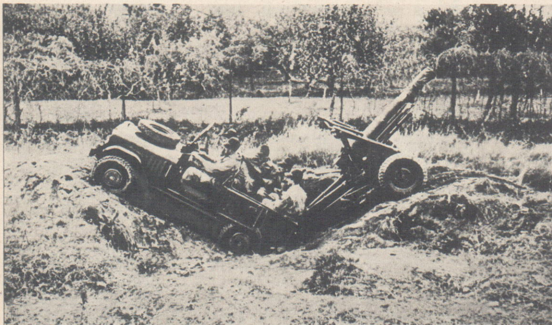
Above: The Gunners may soon be getting this air-portable Italian 105 mm howitzer shown here undergoing tests in Italy. It can be dismantled and carried by mulepack, flown in three sections by helicopter, or broken down into 30 parts and manhandled.
