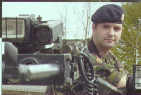
Me and my Wheelbarrow: SSgt Simon Rolls with a Mk8 remote-controlled vehicle used by 621 EOD Sqn personnel when approaching devices
