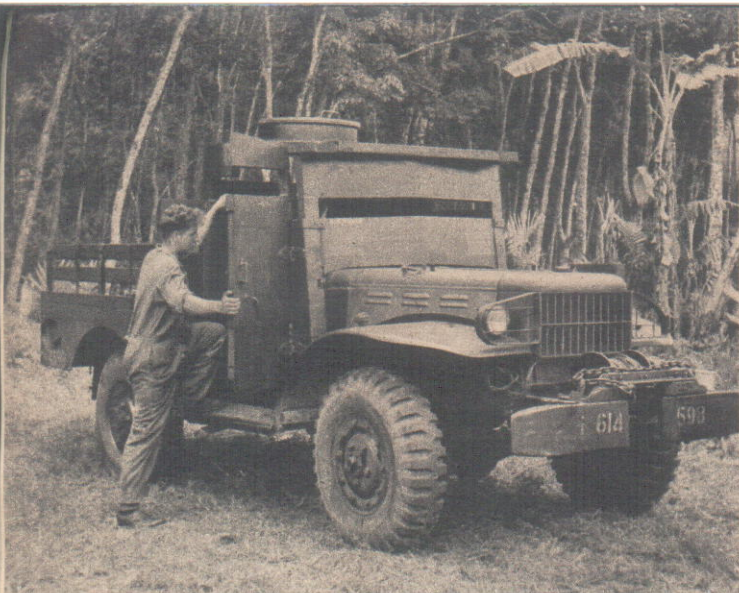
Armoured trucks used by the KOYLI: (above) a 15-cwt converted by REME, and (right) a three-tonner. Note rifles protruding from apertures, side and front.
