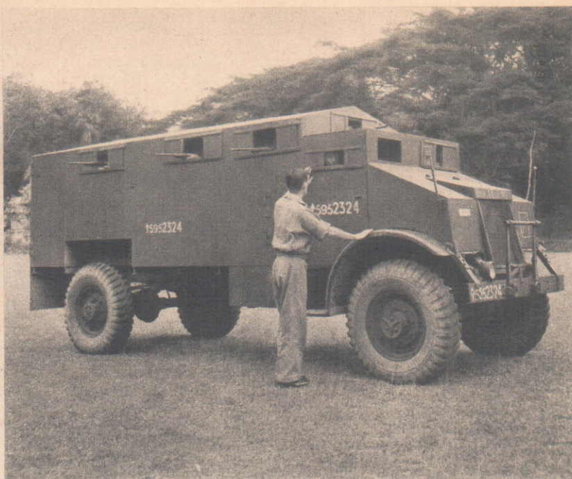
Armoured trucks used by the KOYLI: (above) a 15-cwt converted by REME, and (right) a three-tonner. Note rifles protruding from apertures, side and front.
