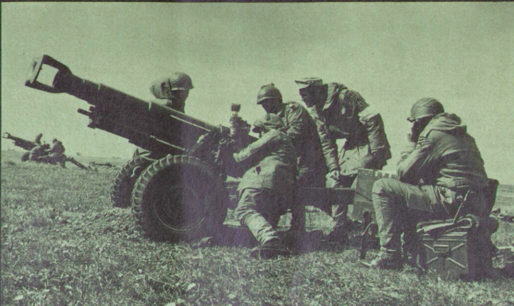
Above: Germans fire their version of the 105mm pack-howitzer. Note the distinctive flash eliminator with which the gun is muzzled.
