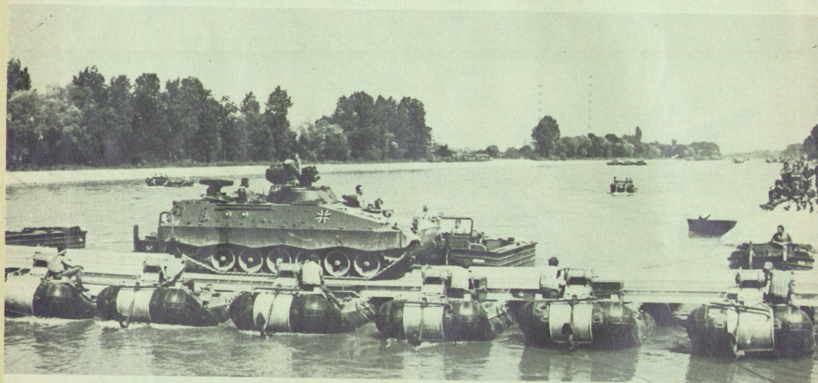
A Bundeswehr Marder AFV uses a German inflatable bridge while men of 9 Squadron and their hosts look on. Below: The British troops master German bridge-building.
