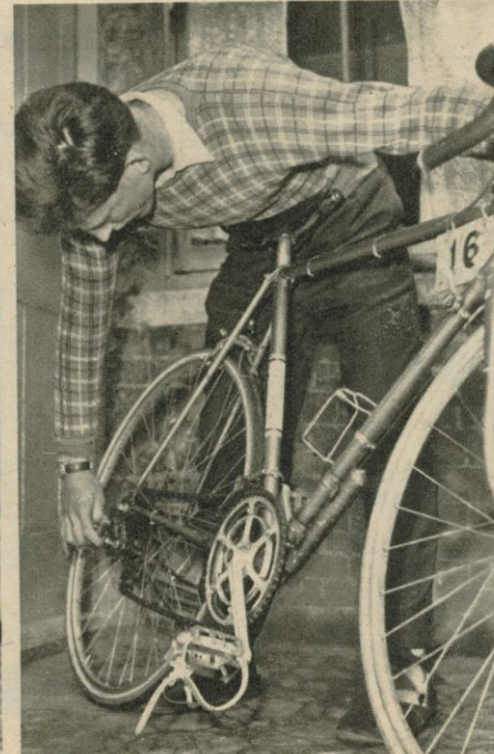
His racing saddle is little bigger than a man's hand. Right: Adjusting the ten gears on his mass-start machine. Note nitrogen pump on down-bar.
