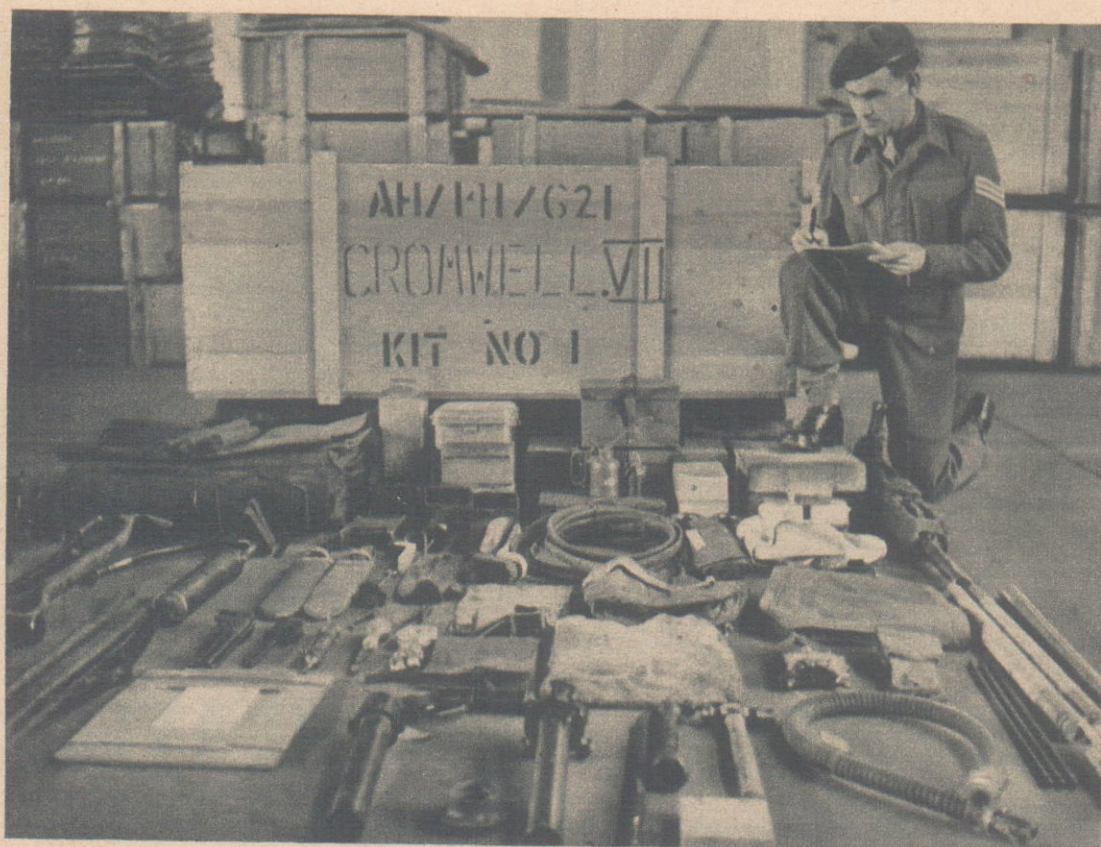
The odds and ends. A tank kit may have between 300 and 400 pieces, every one of which must be checked before the tank is issued.
