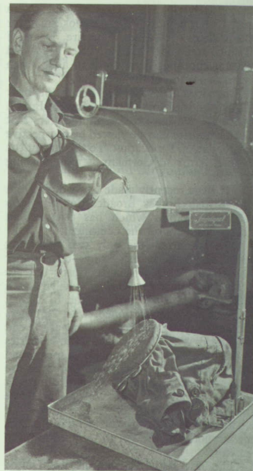
Above: A water repellency test. Combat suits are checked by this method after being reproofed. Half a pint of water poured into the funnel represents three hours steady rainfall. A soldier can expect to stay dry for just this long.
