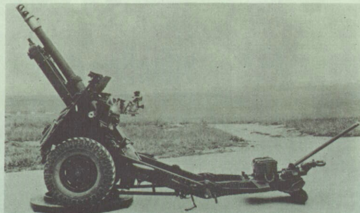
Right: The hinged trail and high elevation earned this mark the nickname "Praying Mantis." The intention was to improve the crest clearance for war in mountain areas.
