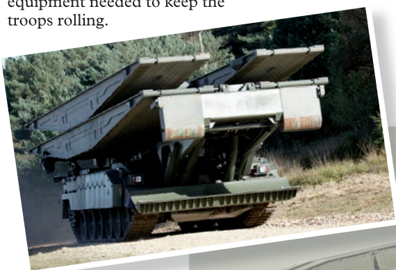
Bridging the gap: Titan, above, carries a close support bridge during a demo in Bovington
