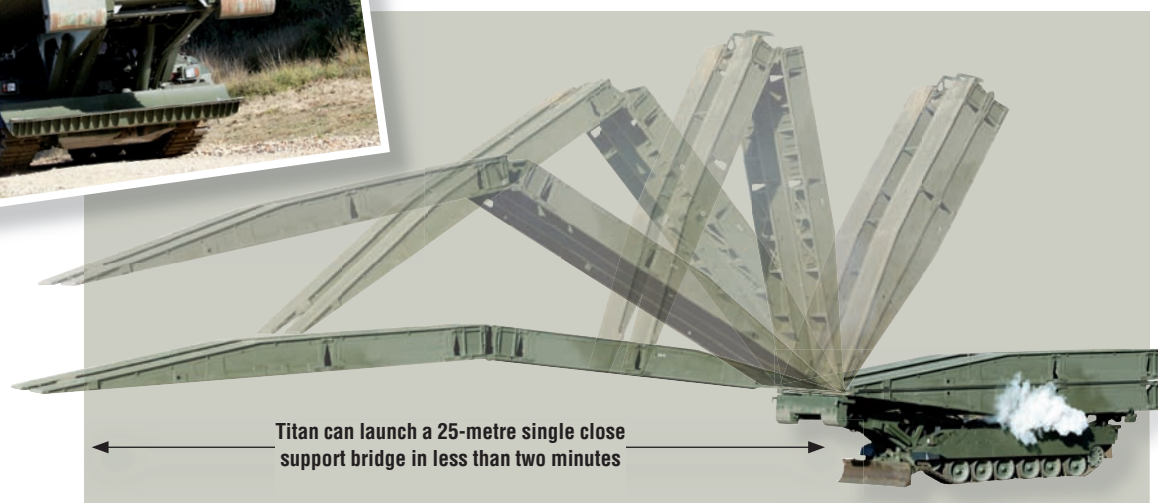
Bridging the gap: Titan, above, carries a close support bridge during a demo in Bovington
