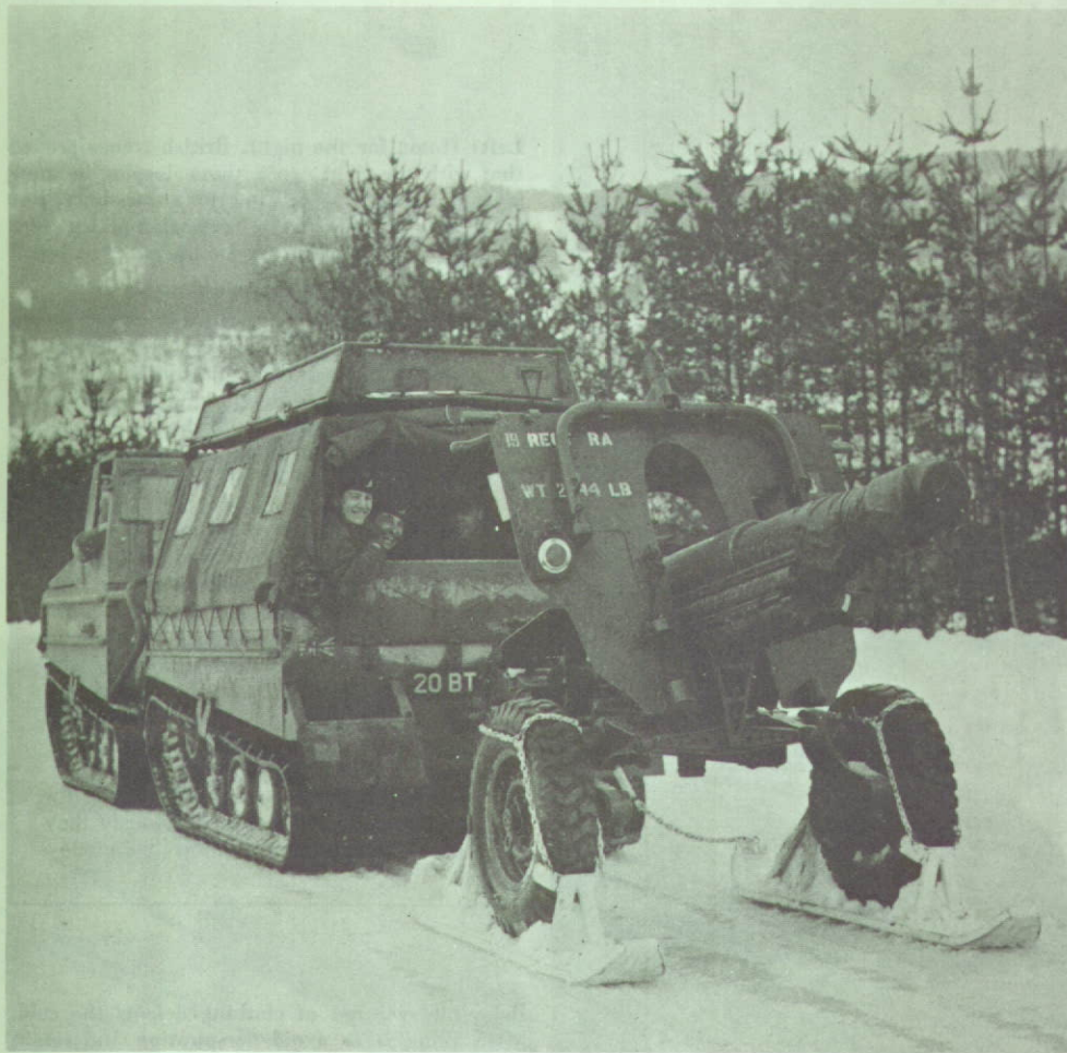
A 105-millimetre pack-howitzer equipped with skis on test with the Volvo over-snow carrier (above). Below: British soldiers on skis surprised the Norwegians and occasionally damaged their own limbs.
