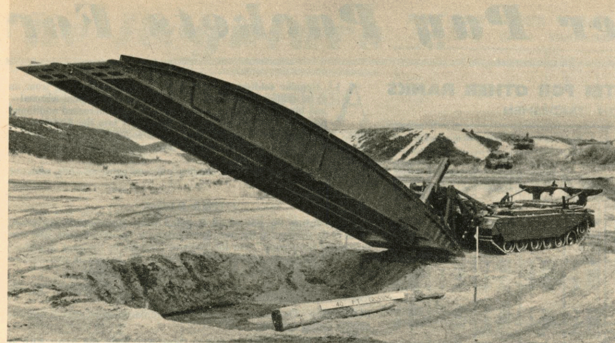
Left: The new Centurion bridge layer. It can span a 40-ft gap and carry a load of 80 tons. The bridge can be launched across an obstacle in three minutes by one man inside the tank.
