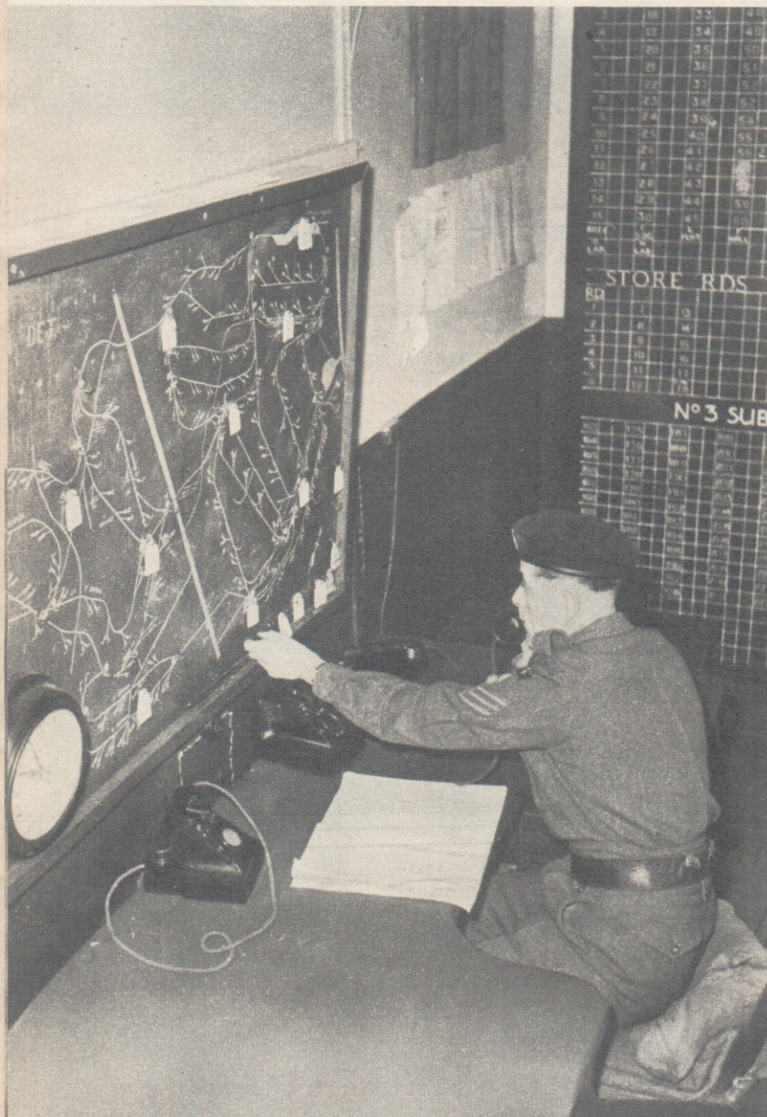
All movement on the Kineton Military Railway is controlled by a regulator board, here being operated by Sergeant J. Hyett, the yard foreman.
