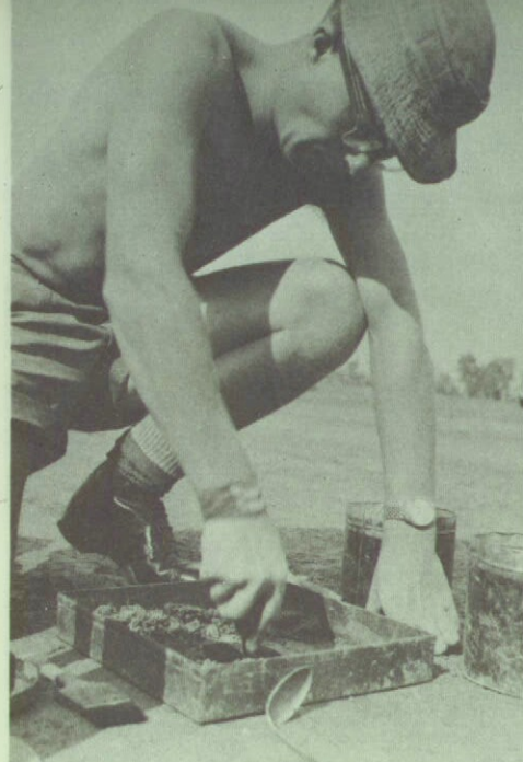
Cpl John Robinson, RE, a soil expert, testing the density of the runway's thick laterite base.
