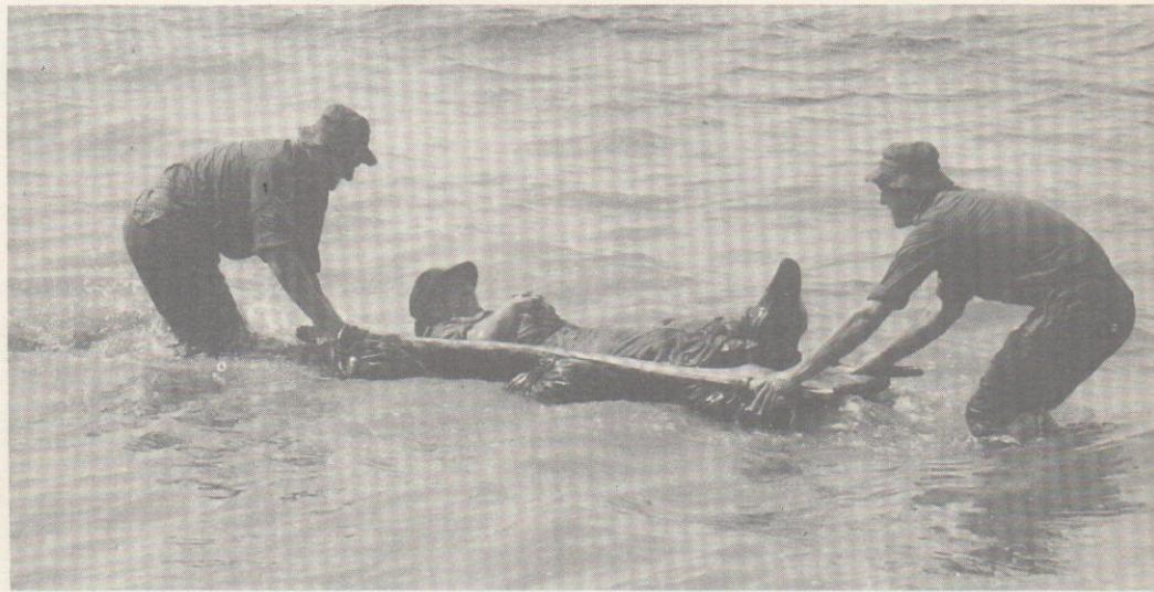
Col Caughley tests a stretcher raft which floats on equipment carefully wrapped in groundsheets.
