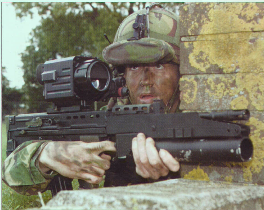
Shape of things to come: WO2 (QMSI) Lea Bates demonstrates FIST technology – an SA80 A2 fitted with a dual waveband sight and 40mm grenade launcher
