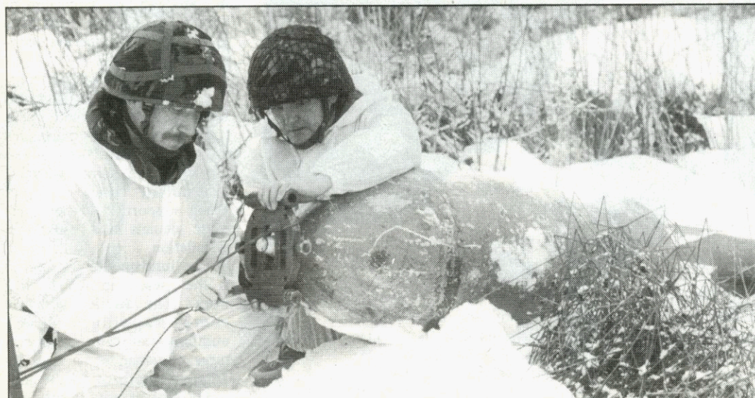
Sgt Dave Percy (left) and LCpl Tomlinson of 49 EOD place an electrically initiated rocket wrench on the fuse of a replica Russian 500kg bomb. The wrench rotates rapidly to unscrew the fuse before it has time to detonate the bomb
