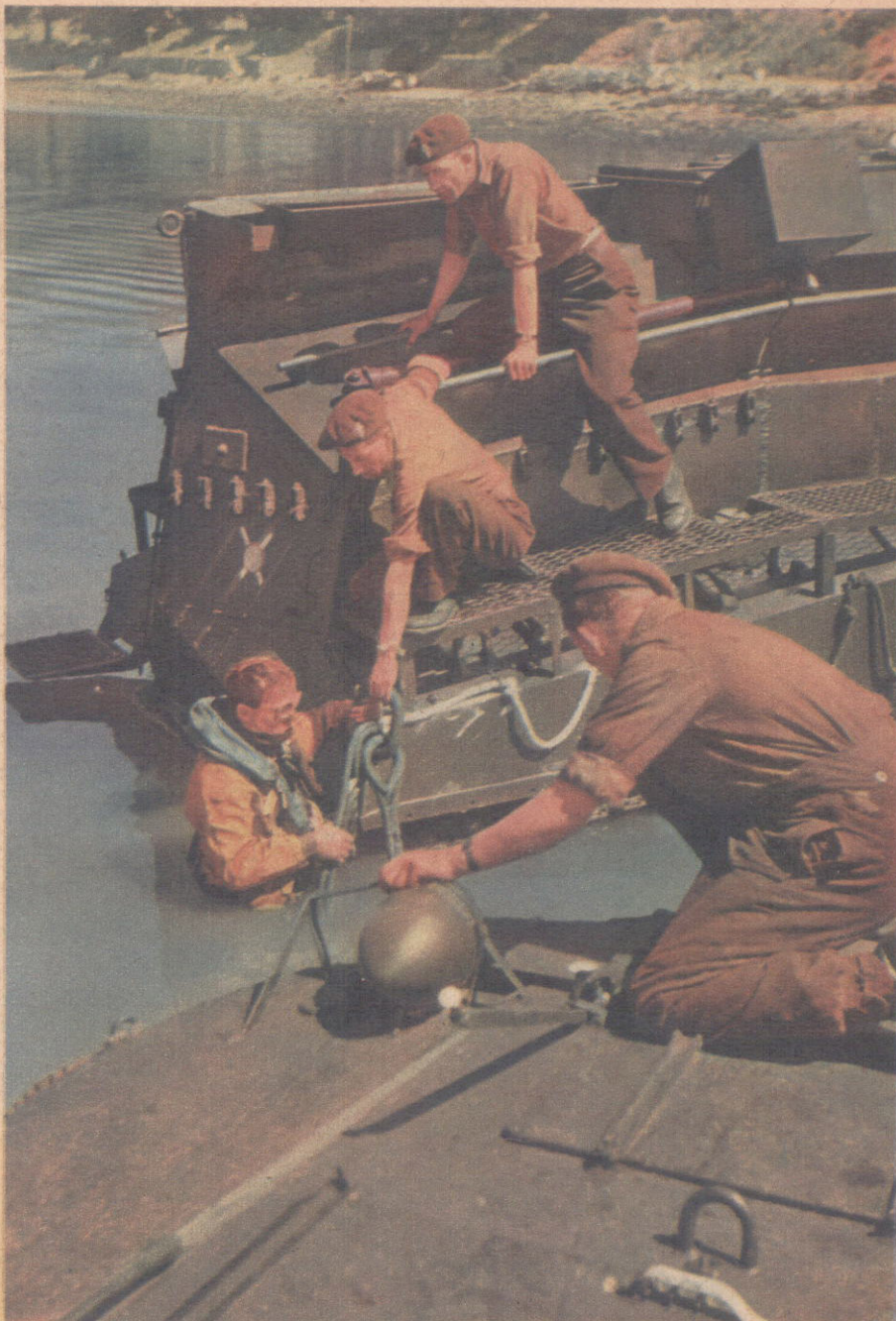
Above: Last-minute instructions for the diver who goes out with the beach armoured recovery vehicle. He inspects sunken vehicles and attaches tow ropes.
