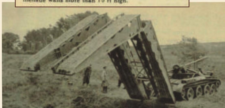
A "Scissors"-type bridge mounted on a tank chassis. The hydraulic ram is closing the bridge to return it to the carrying position
