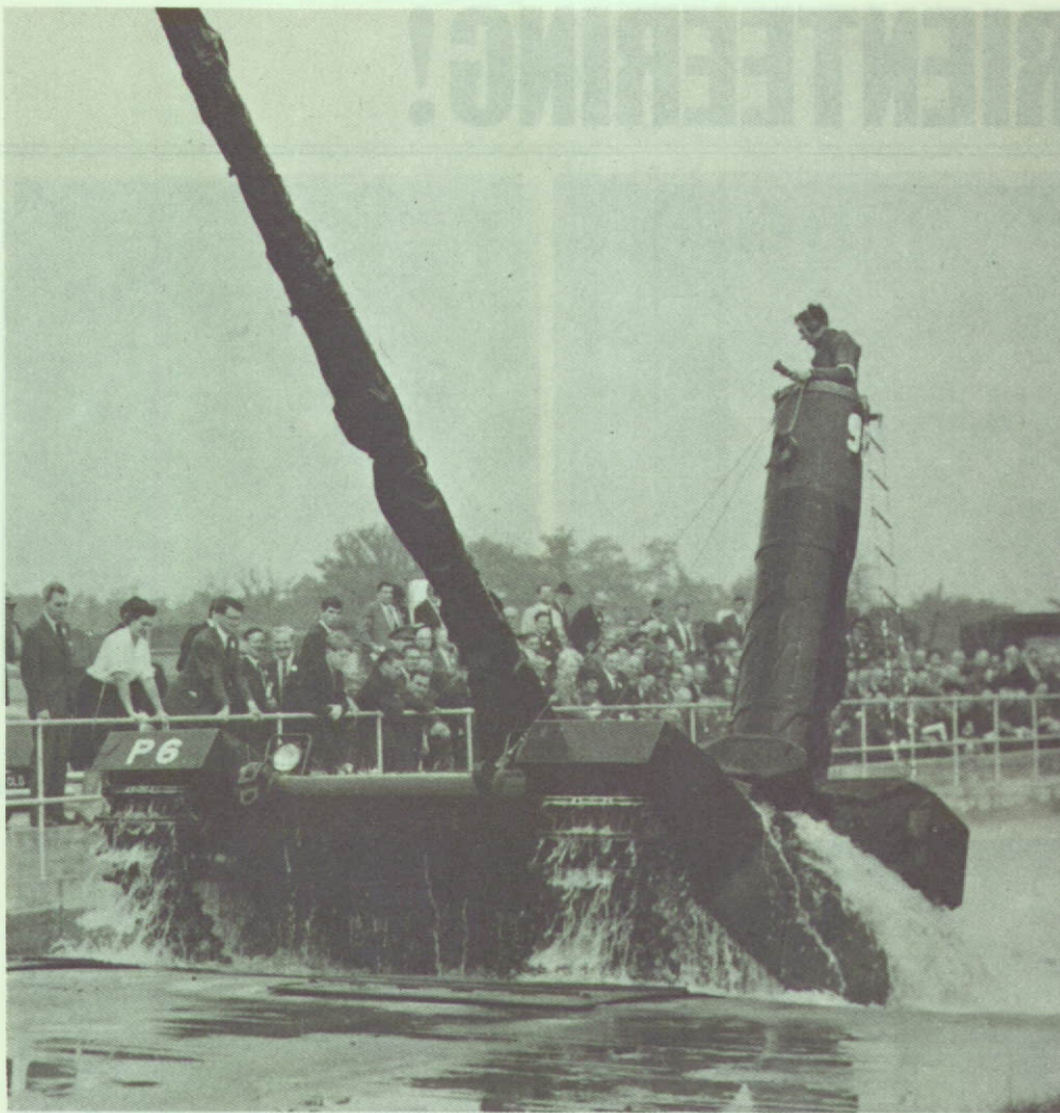
Left: A Chieftain tank, fitted with snorkel, emerging after wading through a 15-foot depth of water.
