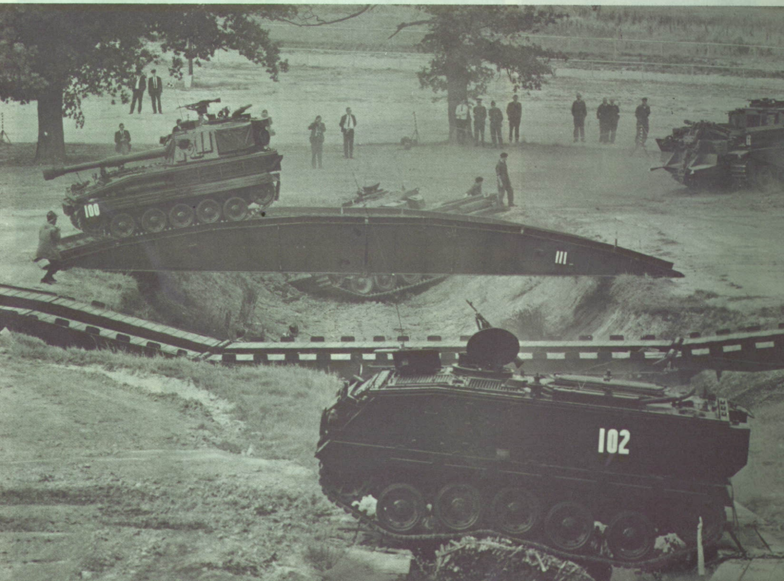
Below: In the foreground FV 432 in the Carl Gustav role crosses a gap bridged by Centurion-laid fascines. Behind, the Centurion Mk V Ark bridge, and beyond that the Class 80 bridge laid by the Centurion Mk V bridgelayer, with Abbot crossing over it. Behind the bridge a "ditched" Centurion about to be winched out by a Centurion armoured recovery.
