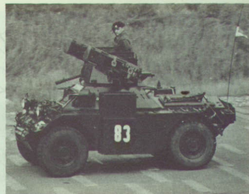
The Daimler Ferret scout car Mk II (above) seen in one of its roles of carrying four Vigilants.
