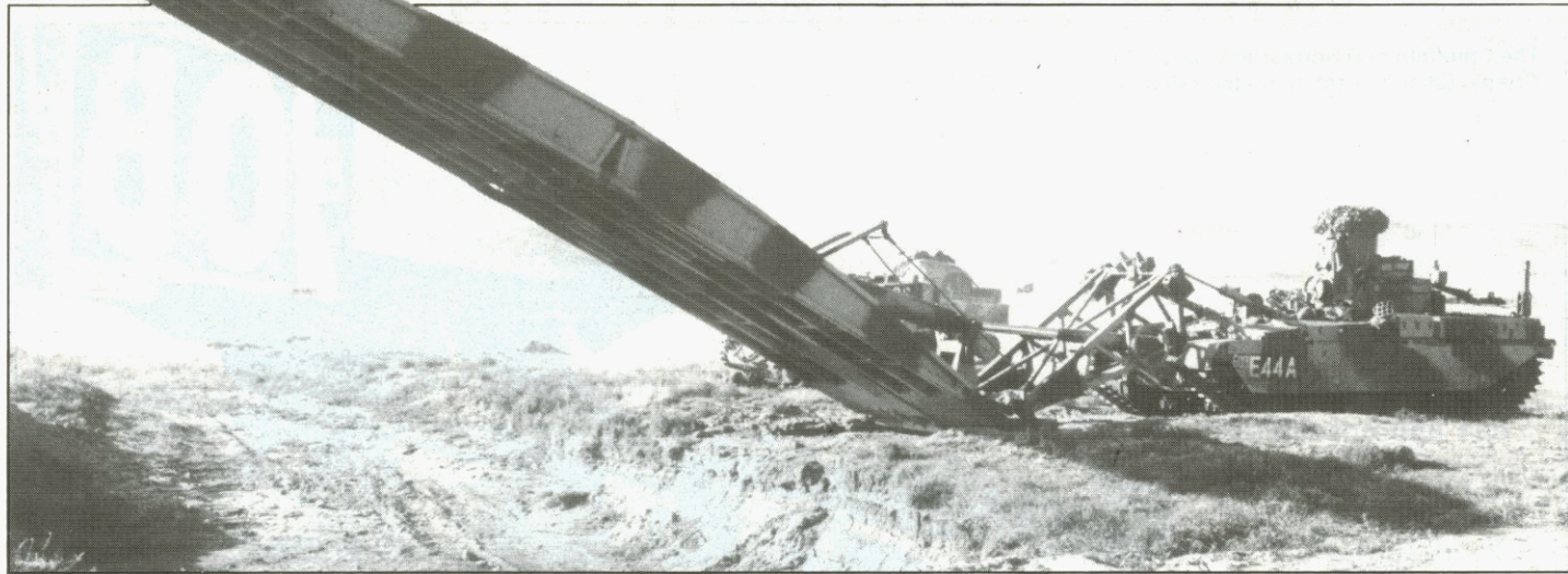
An AVLB of 21 Engineering Regiment, supported by tanks of 4 RTR, prepares a river crossing
