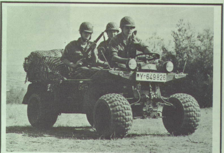
Both the Belgian and German battalions tested two small cross-country load carriers during the exercise. Above is the German Kraka which folds in two for para-dropping and carries \frac{3}{4} ton and below is a Belgian three-wheeler capable of carrying four men.
