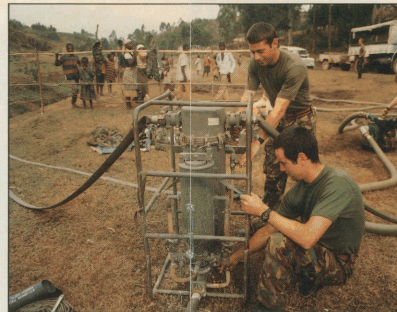
Spr Ian Worland (standing) and Spr Colin Campbell check machinery at the reverse osmosis plant, which provides clean water
