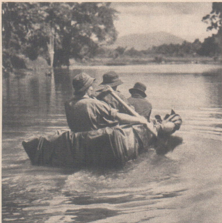
Three soldiers man a river craft made by wrapping ground-sheets tightly round a bamboo frame bound with vines. The paddle is a stout stick with slats pushed through to make a blade.
