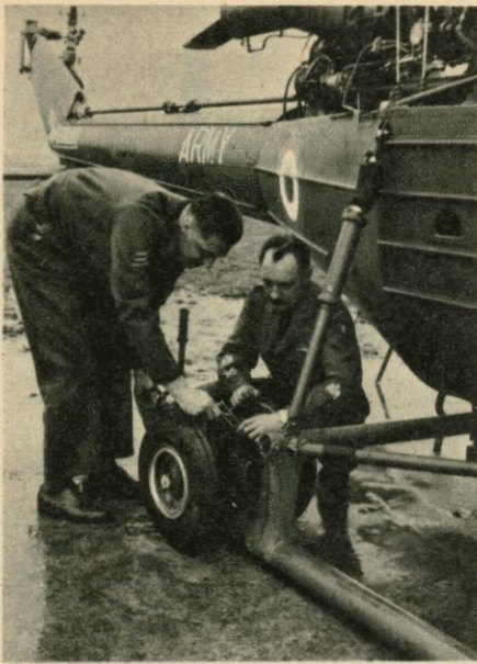
Fitting the ground handling wheels to the Scout's skid landing gear. Flotation bags or conventional wheels can be fitted as alternatives to the skidgear.
