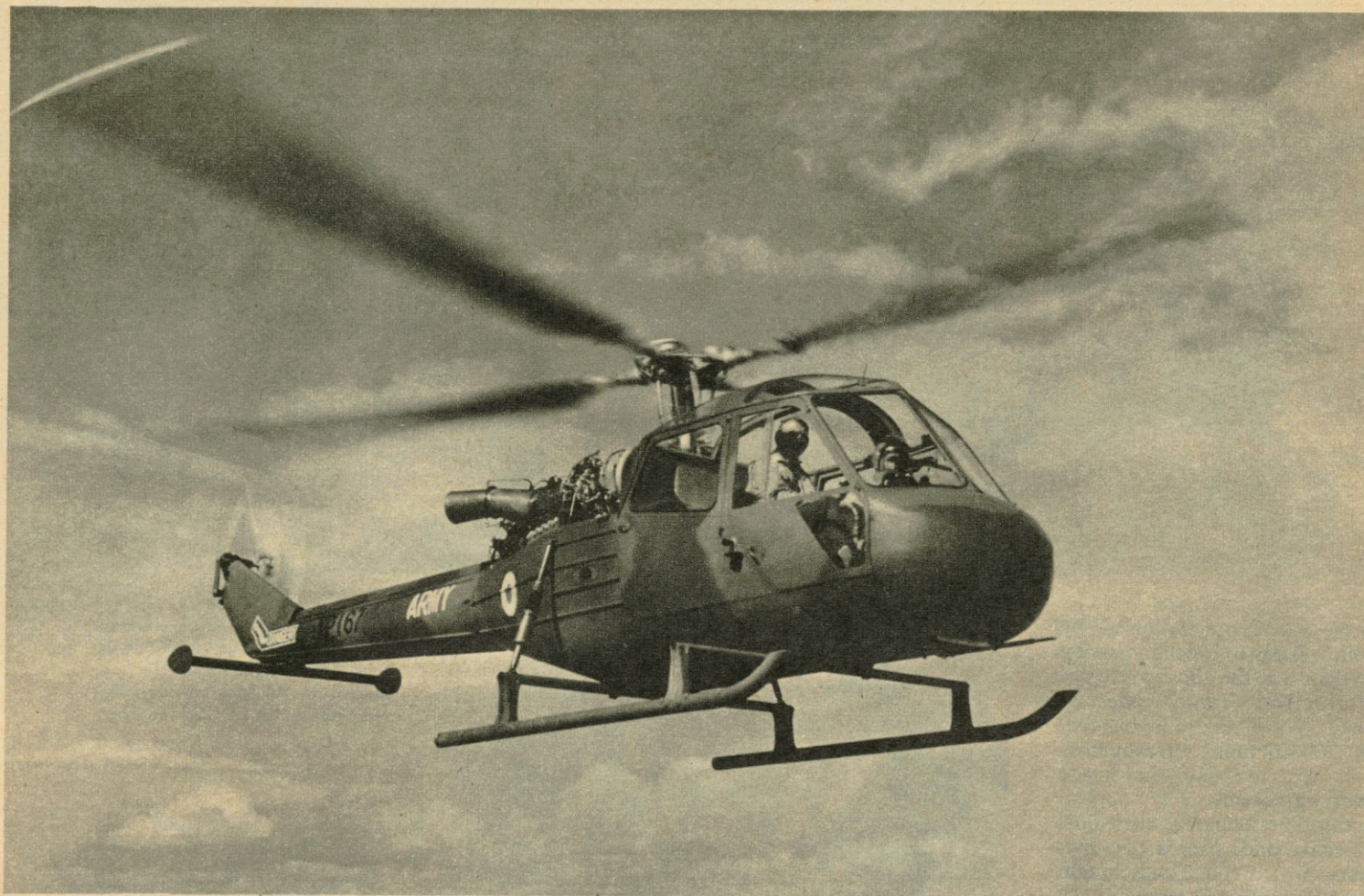
Like the French Alouette , the Scout has a skid undercarriage and a gas turbine engine which is completely in the open and therefore much easier to service. A bench seat behind the pilot can be folded back for freight.
