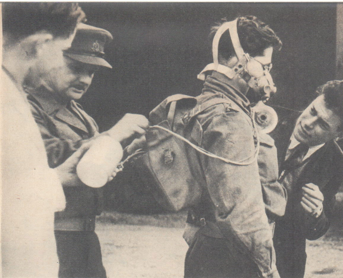
While Major J. M. Adam removes air samples, the inventor, Mr. H. S. Wolff, checks temperature shown by a thermometer on the air-flow meter.
