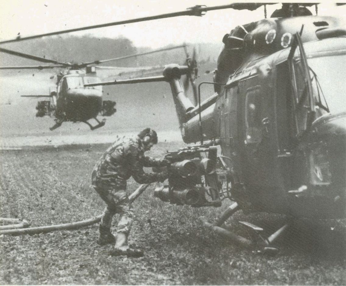
Above - The rapid refuelling techniques employed by members of the ground-support staff of 3 Regiment, Army Air Corps provided a quick turnaround between missions for a gaggle of Lynx helicopters from 653 Sqn AAC
