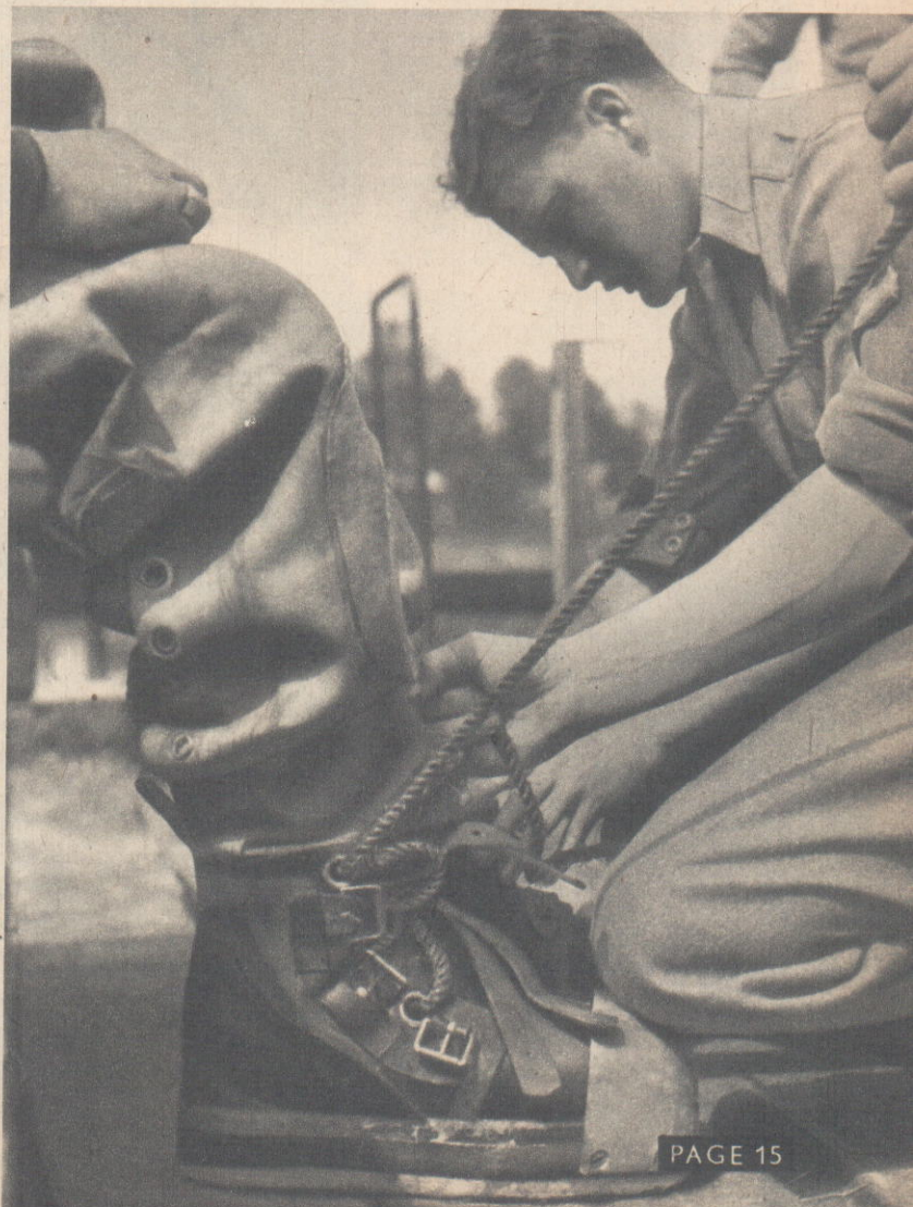
Below: Divers' bootlaces are made of thick tarred rope. The boots, capped with brass, weigh 19 pounds each.
