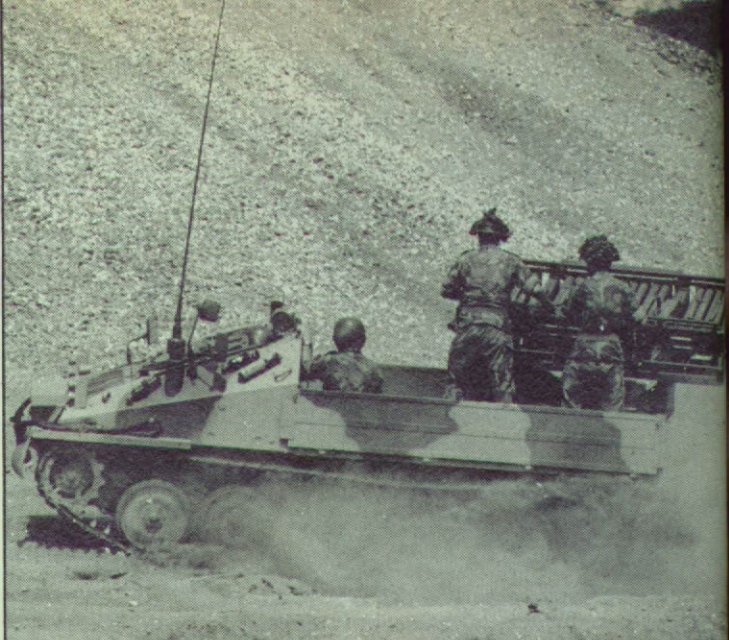
Streaker and its aerial mine-dispensing facility, Ranger.
