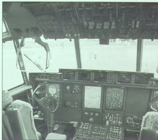
Heads up: Liquid crystal displays and head-up screens convey vital data to pilots
