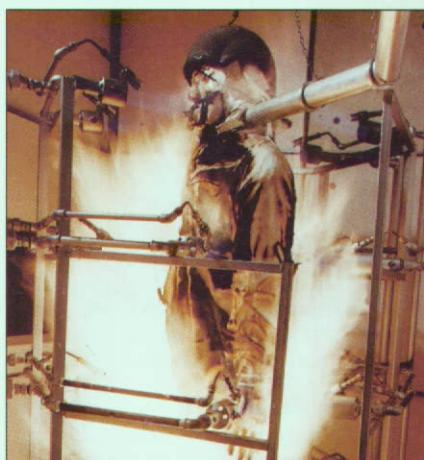
Flash fire: Flame-retarding garments are tested to destruction in the Defence Clothing and Textile Agency labs. Synthetic fibre suits for those particularly at risk from flash fuel fires are now able to protect wearers from the fierce heat for up to five seconds, long enough to allow a trained person to escape from a cockpit or a vehicle, or for fire extinguishers to be activated.
