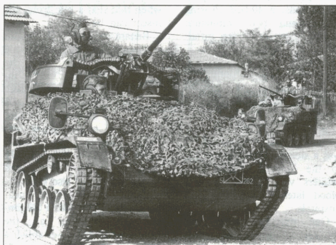
The German 263 Airborne Battalion is equipped with Wiesel. This version of the airportable armoured vehicle has a 20mm cannon
