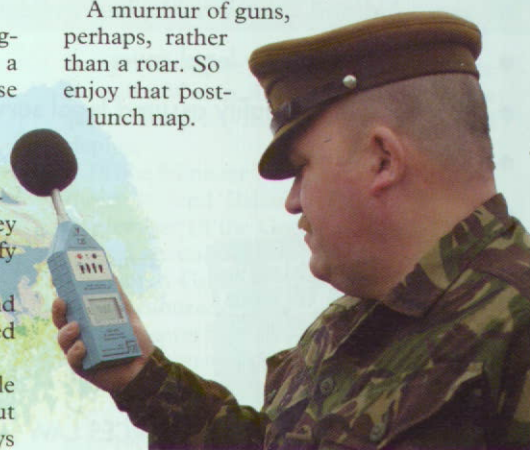
Monitor: WO2 Les Fortey checks noise levels with a hand-held sound level meter
